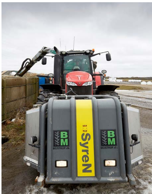
Figure 4.2 | Farmers must mix manure before spreading it on farm fields and can add acid just before to reduce ammonia emissions in the field.
